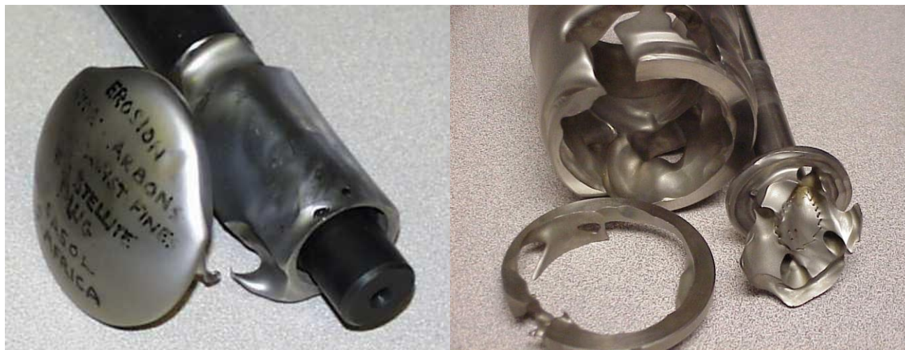
Figure 10. Flashing erosion damage in control valve trim.
