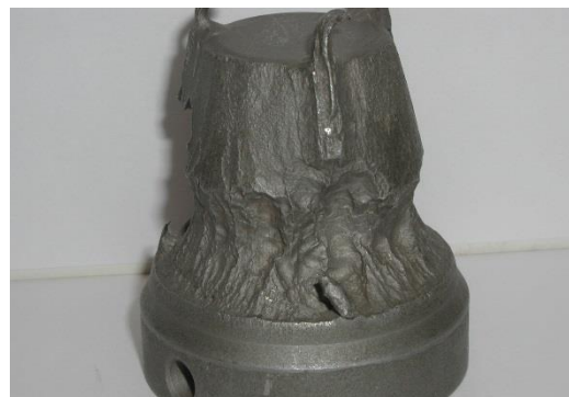
Figure 1 Cavitation damage on valve plug
