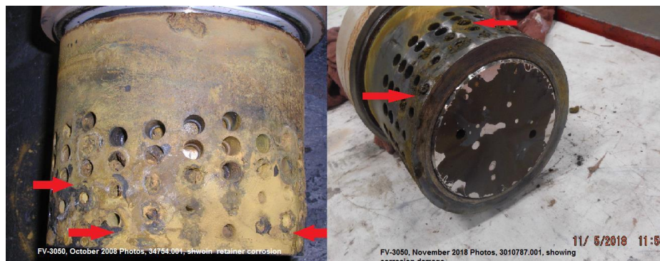
Figure 6. Plugged Anti-Cavitation trim
