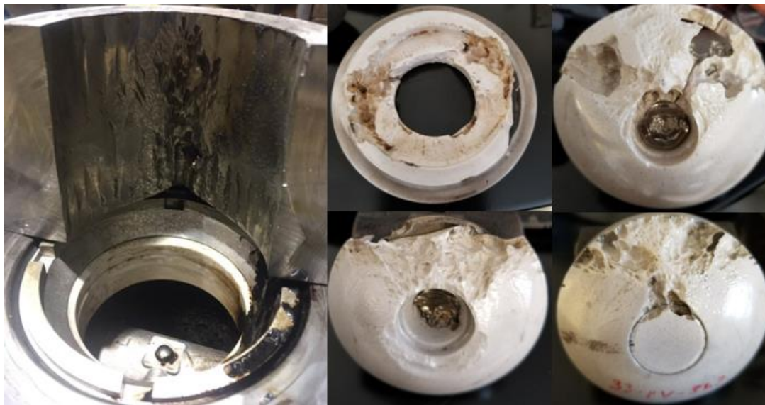
Figure 8. Cavitation damage on ceramic trim.
